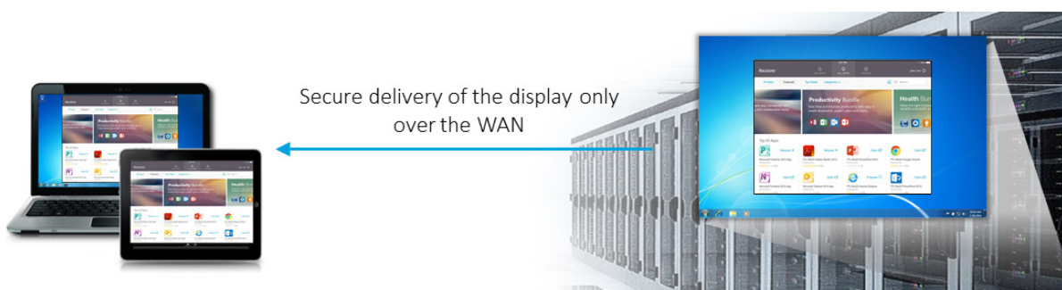
Figure 1 - Windows workloads run in the datacenter and only the display is sent to the user.
